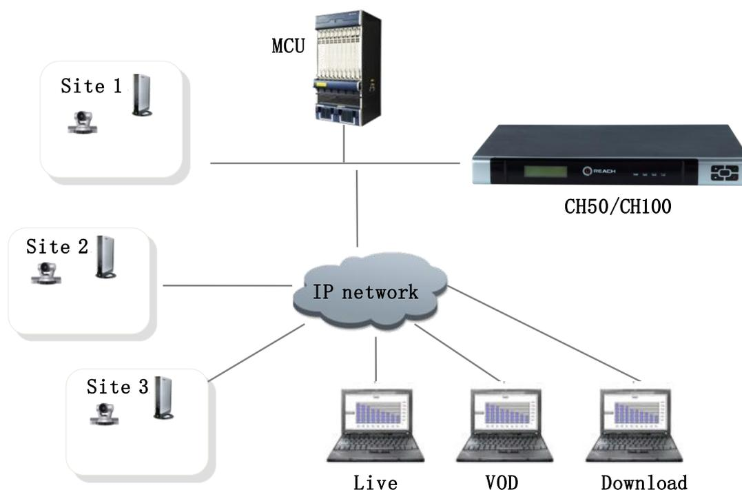
The recording and streaming server, MCU, and video conferencing terminals are in the same network and use H.323 protocol for mutual communication. Upon adding to a conference, the recording and streaming server enables the recording port to start and stop recording.
