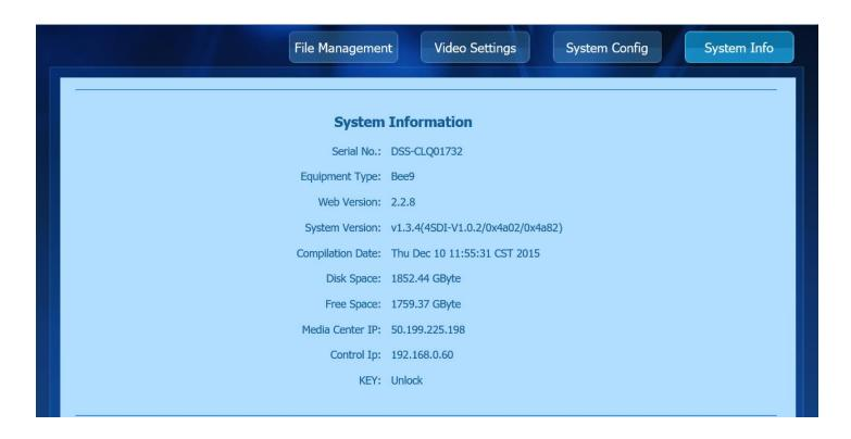
The system info page is where we started when we logged in to the Bee9 as an administrator. The information on this page is valuable to the IT professional, and integrators, as it completely describes the Bee9 physically, and where it is on the LAN. After preparing the Bee9 for deployment, this page allows users to confirm the equipment is ready to be interfaced with the Director application, and the Kite application to continue the process of configuration.
